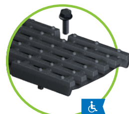
Ductile iron elongated bar grating MW 29/13 – NW 100 & 150 MW 25/13 – NW 150 up to class D MW 22/13 – NW 150 & 200, up to class E 4 point bolted only available in cast iron edge
