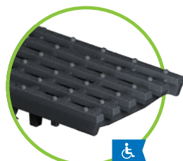
Ductile iron elongated bar grating MW 29/13, class C or class D for NW 100 to 200
