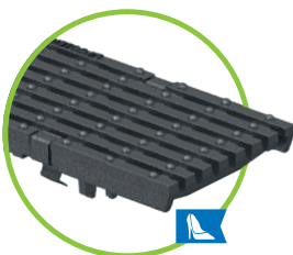
Ductile iron elongated bar grating MW 29/6 narrow SW, cl. C for NW 100
