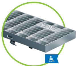
Mesh grating, cl. B – galvanized steel and class C galvanized steel / stainless steel, MW 30/10, for NW 100
