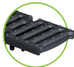
Ductile iron slotted grating SW 14/100, cl. E for NW 100
