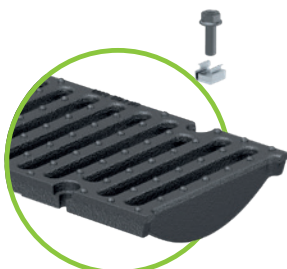
Ductile iron slotted grating SW 14/100, 14/150, 14/200 for NW 100 to 200 class F, 4 point bolted
