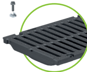
ductile iron slotted grating SW 16/140, class F 900 4-points bolttable
