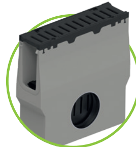
Sump unit, one-piece, incl. ductile iron grating, silt bucket, outlet DN 150
