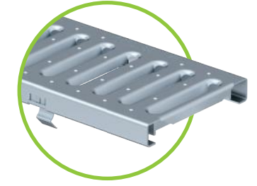
3. Slotted grating SW 0.31" x 3.15" (8x80 mm) cl. C galvanized or stainless steel V2A for NW 100
