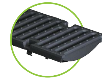
8. Ductile iron slotted grating SW 0.55" x 3.94" (14x100 mm) SW 0.55" x 5.91" (14x150 mm) SW 0.55" x 7.87" (14x200 mm) for NW 100 to 200 cl. E with fix self-locking system
