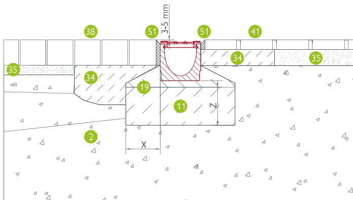
BG-FILCOTEN® light NW 100: pavement – pavement covering, class A – C
