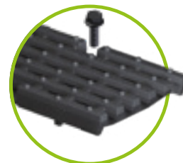
ductile iron elongated bar grating MW 29/13 – NW 100 & 150 MW 25/13 – NW 150 up to class D MW 22/13 – NW 150 & 200, up to class E 4 point bolted only available in cast iron edge
