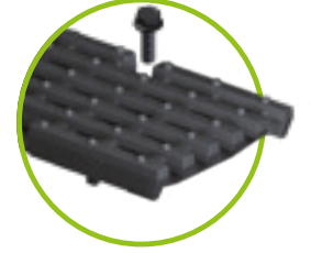
ductile iron elongated bar grating MW 29/13 – NW 100 & 150 MW 25/13 – NW 150 up to class D MW 22/13 – NW 150 & 200, up to class E 4 point bolted only available in cast iron edge
