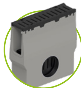
Sump unit, one-piece, incl. ductile iron grating, sediment bucket, outlet DN 150
