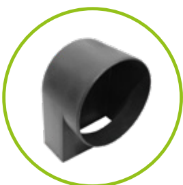
Odour trap for sump unit for retrofitting Ø 100/150 Installation: Insert the odour trap from the inside and connect with the sewage pipe.
