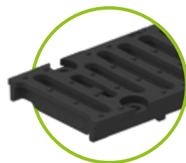
Ductile iron grating SW 16/120 and/or 16/220 – class F 4 point boltable, for NW 100 and 200
