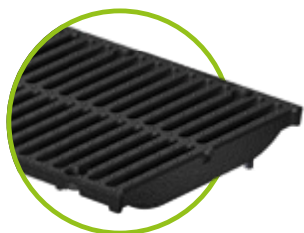
Ductile iron slotted grating SW 18/215, class E 4 point boltable
