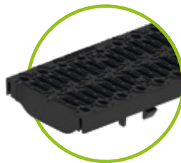
Plastic slotted grating SW 8/40 and/or 10/58, class B and class C plastic PA6 for NW 100 and/or NW 150
