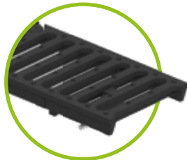
Ductile iron slotted grating SW 16/120, 18/120, 18/170, class C or class D for NW 100 - 150, SW 18/220, class D for NW 200, SV or 2-point bolting
