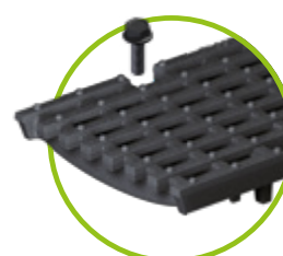
Ductile iron longitudinal bar grating MW 25/13 up to class D MW 22/13 up to class E, 4-point bolted only available in cast iron edge
