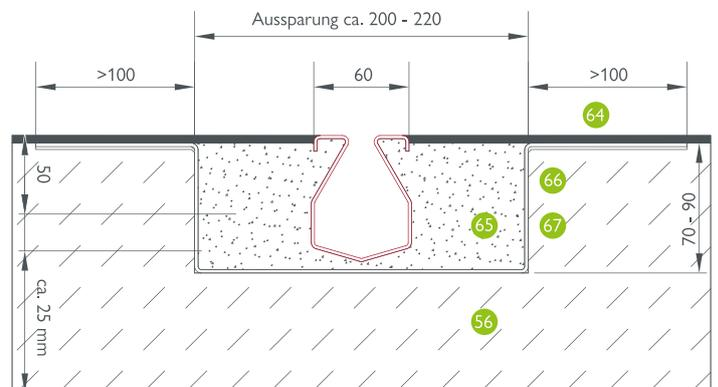
BG-FLEX omega, SW 16, Beschichtung, Kl. A – C
